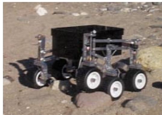
Fig. 2 The rover test bed moving on rocky rough terrain
