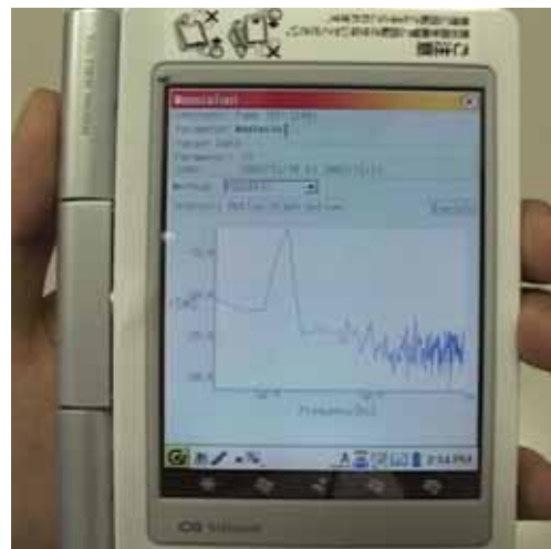
Fig. 6 Result of spectrum analysis using FFT on MASSIA Tool
