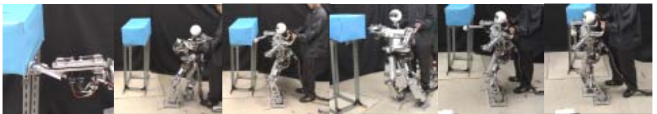
1. Search and touch obstacle. 2. Whirl back. 3. Confirm obstacle. 4. Side walk. 5. Reconfirm obstacle. 6. Walk forward.
