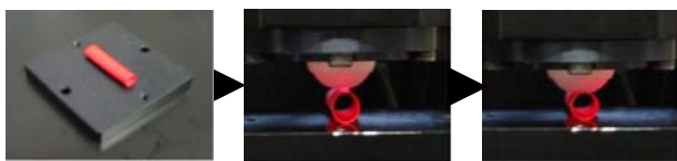
Fig.10 The measured object which cut into the balloon at 0.5 mm
