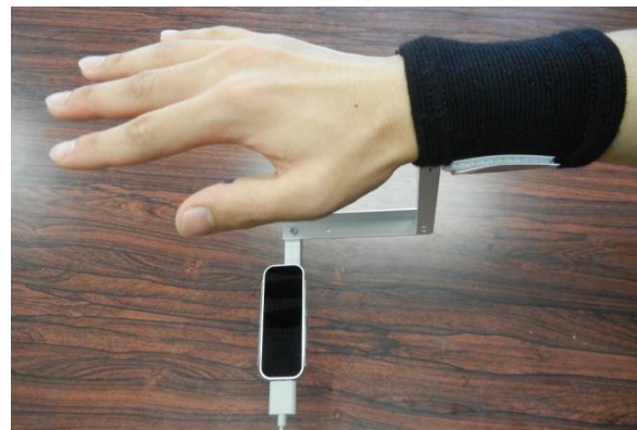
Fig.3 Implement of Leap Motion on the wrist
