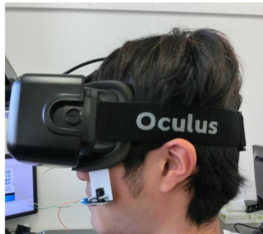
Fig.12 Installation of the sensor to HMD
