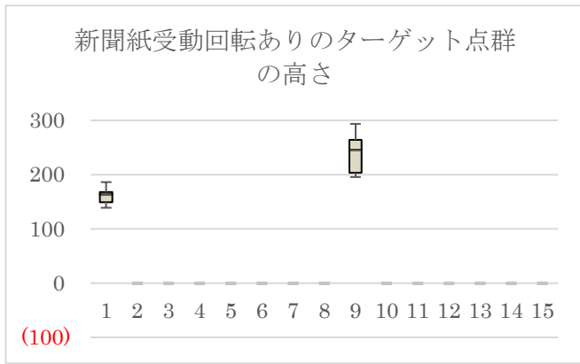
Fig.15 The distance of reconstructed target points from the estimated floor plane with passive joint camera with newspaper.
