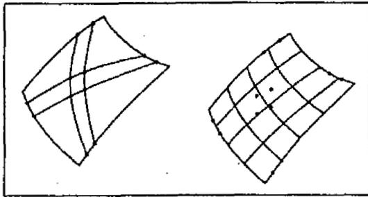
Fig. 5 Smoothing scatter data points to surface, the maximum deviation between point to the surface is 0.02, for the smoothness weight 0.01 in both u and v parameters directions.
