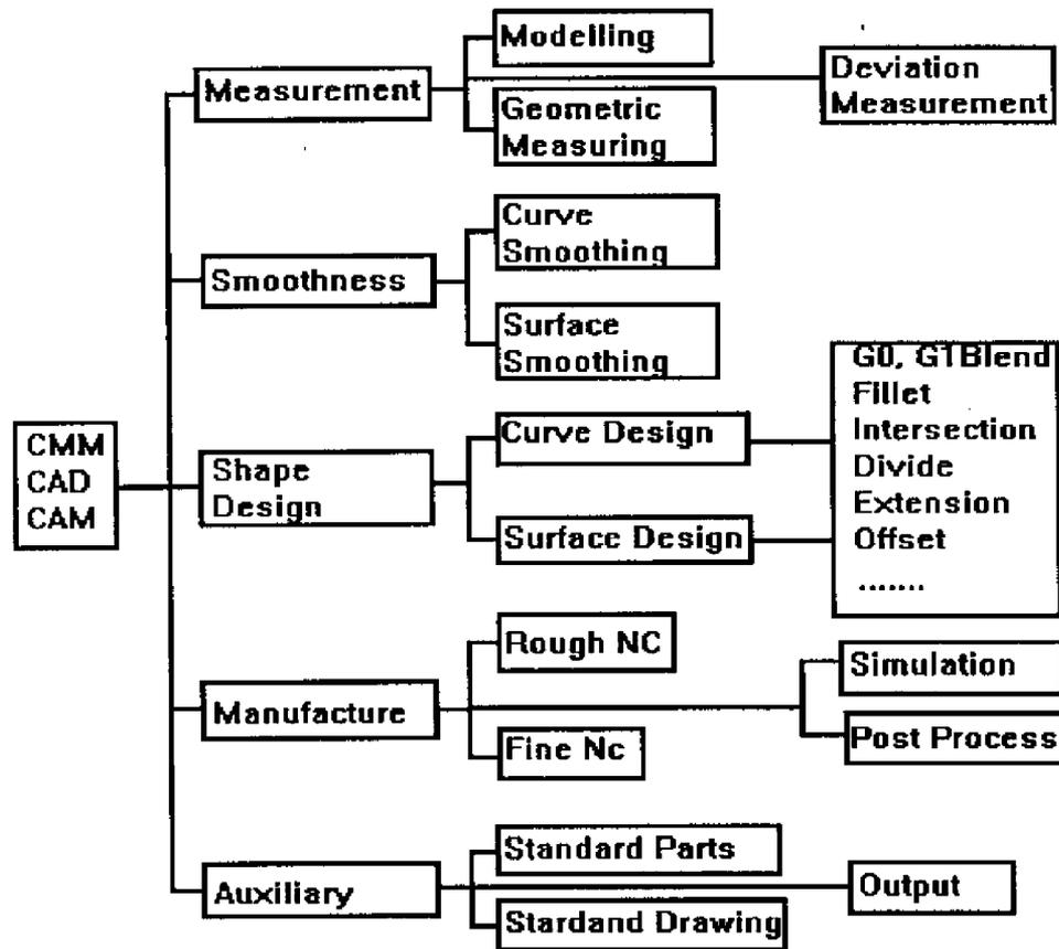
Fig. 2 The layout of the system
