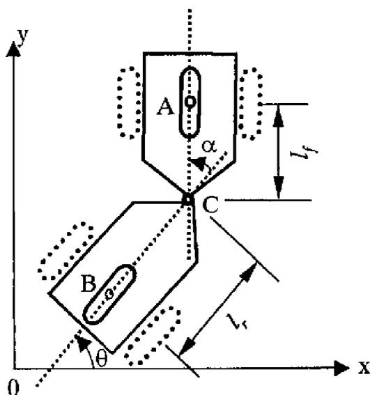
Fig. 1. Schematic diagram of articulated frame tractor
