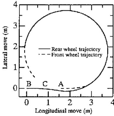
Fig. 5a. Trajectories of front and rear wheels of AFSV when the wheelbases are of equal lengths
