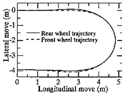
Fig. 7a. U-turn of AFSV when the length of both wheel bases are same
