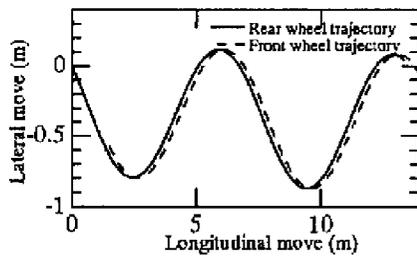
Fig. 8. Slalom motion of AFSV when the length of both wheelbases are equal
