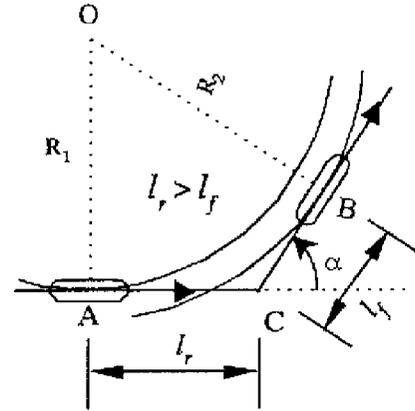
Fig. 3b. Off-tracking condition
