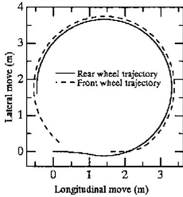
Fig. 6a. Trajectories of front and rear wheelbases of AFSV when rear frame is larger than front frame
