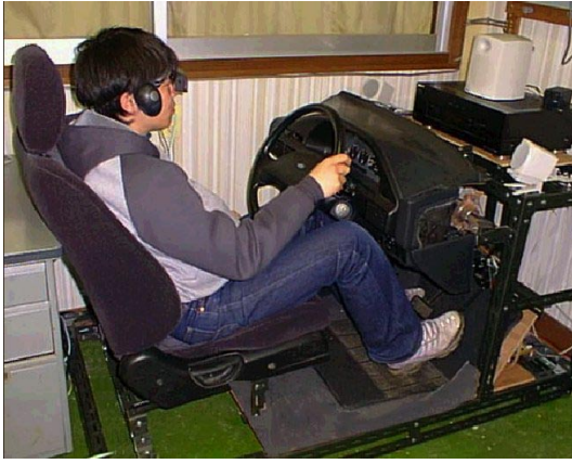
Fig. 3 Driver's seat with force-feedback steering wheel.
