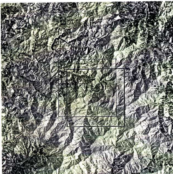
Fig. 3 Satellite image corrected according to system information. Displacement (36 pixels and 31 lines) is found by searching maximum spatial correlation in square regions.
