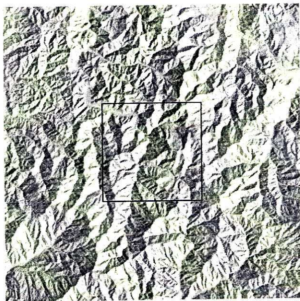
Fig.2 Simulated image of direct solar irradiance from digital elevation model and solar position. Digital numbers in square region are used for the calculation of spatial correlation
