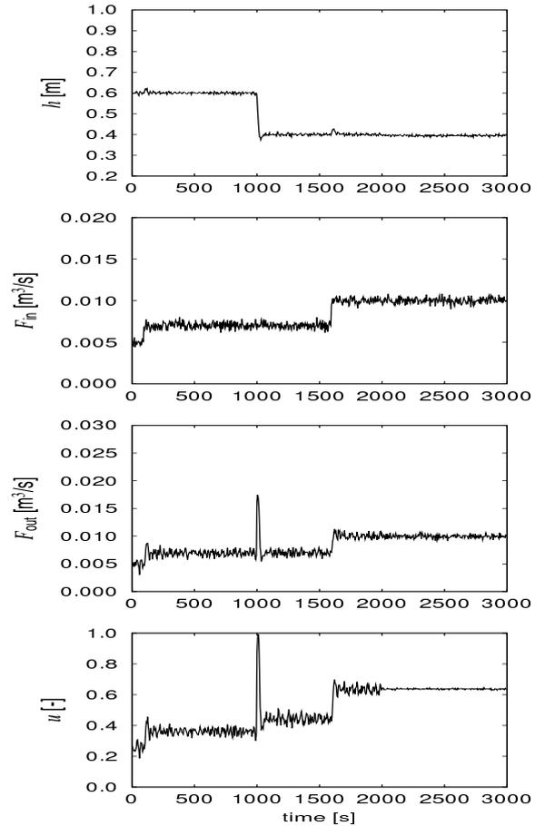
Fig. 7 Faulty operation (valve stuck)
