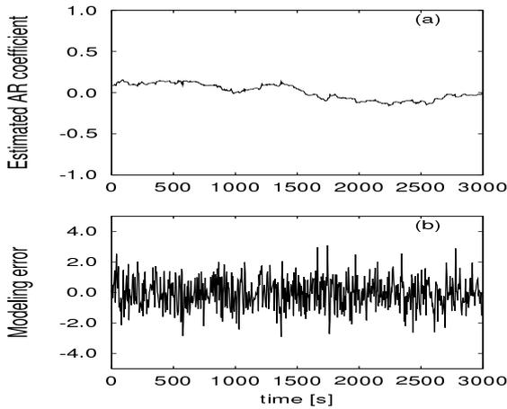
Fig. 6 Estimated AR coefficient and modeling error for the residual
