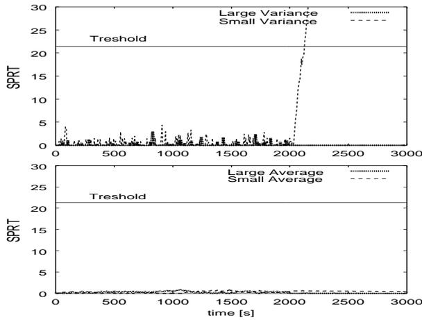
Fig. 9 Result of Fault Detection by SPRT
