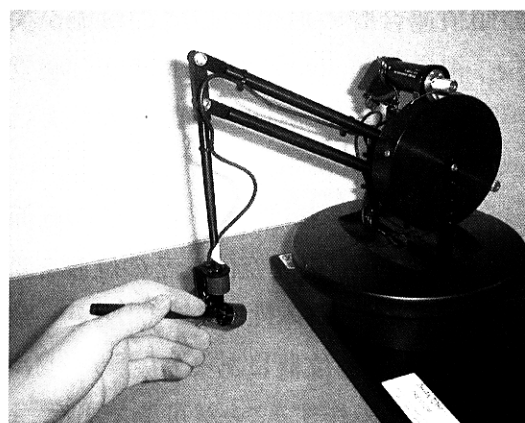
Fig.6 Force feedback device (PHANToM).
