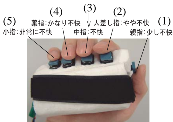
Fig. 4 Evaluation switch of ride comfort. The stronger the subject feels uncomfortable, the bigger the selected number of the button is.
