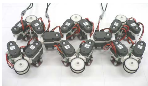
Fig.4 Peristaltic Crawling Robot Using Servo motors
