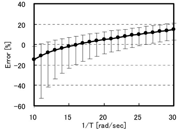
Fig.5 Effect of Cut Off Frequency on the Estimated Calculation
