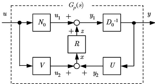
Fig.1 Left co-prime factorization based description of  $G_p(s)$
