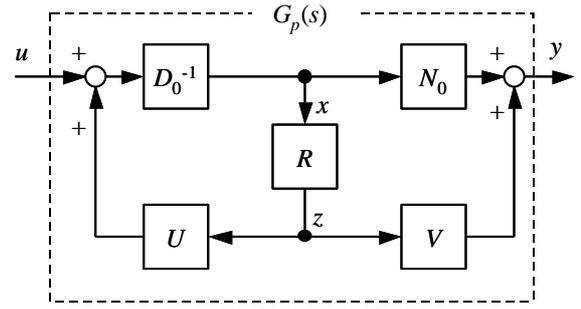
Fig.3 Right Co-prime Factorization Based Description of  $G_p(s)$
