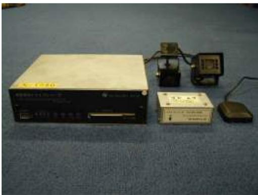
Fig.2 Emergency Lifesaving Drive-Recorder
