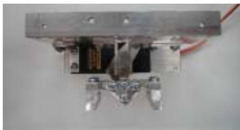
(c) the sole mechanism without sole plate
