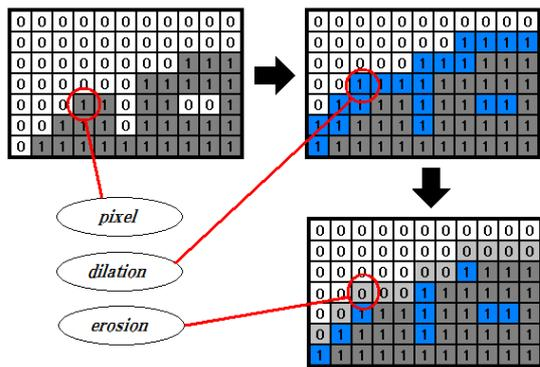
Fig. 2 Dilation and erosion
