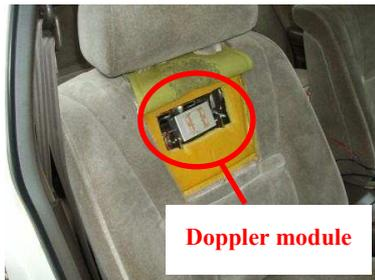
Fig.2 Equipped with Doppler module the car
