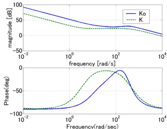
Fig. 7 Bode Diagram of Controllers :  $K_0$  and  $K$
