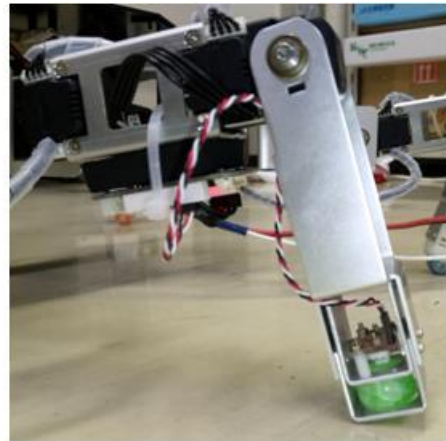
Fig.7 Force sensor attached to robot's foot
