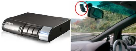
Fig.1 Drive recorder (DR-9100) installation (left: main unit, right: camera)
