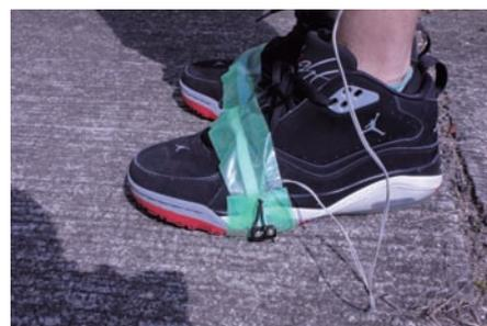
Fig. 6 Attaching the limit switch
