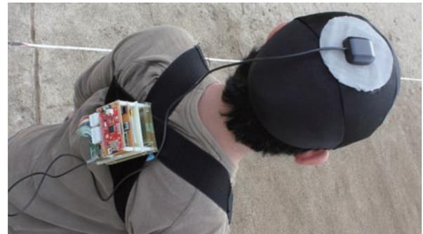
Fig. 5 GPS antenna is mounted on the top of head
