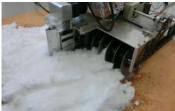
Fig.6 Compacting experiment using shaved ice
