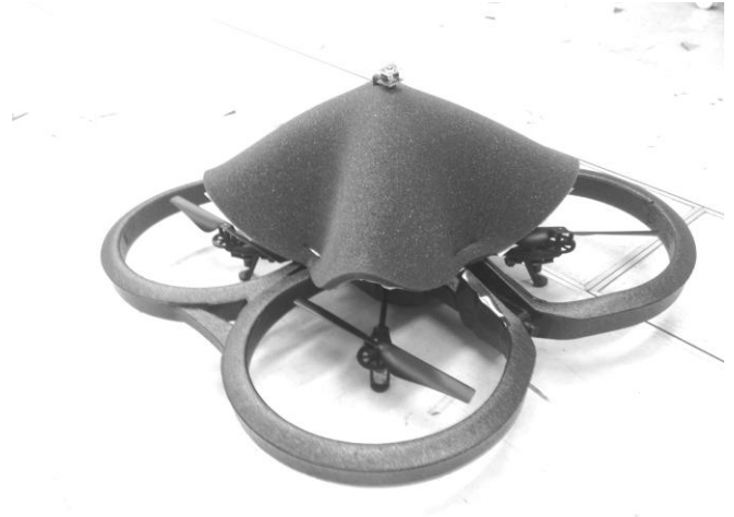
Fig. 5 Flying object subjected with a hull for avoiding wind from propellers
