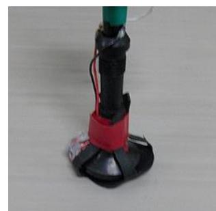
Fig. 5 Pressure sensor attached
