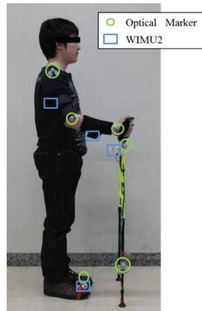
Fig. 8 Installation of 4 WIMU2 and the optical markers.
