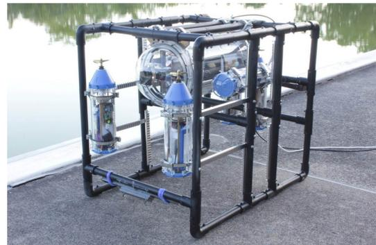
Fig. 1 Prototype of proposed underwater robot
