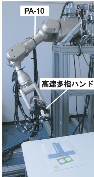
Fig. 8 Robot arm with a multi-fingered hand
