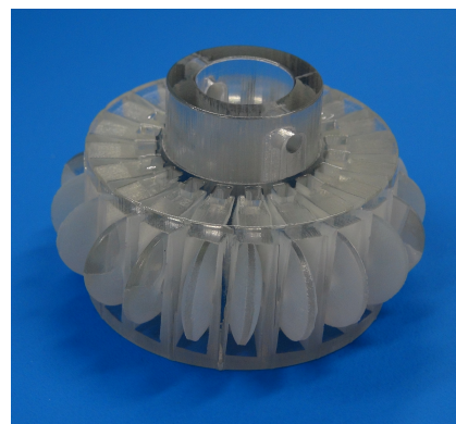
Fig. 4 Worm wheel with flat passive rollers
