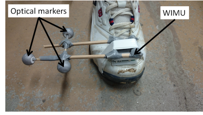
Fig. 8 WIMU with reflective markers mounted on shoe
