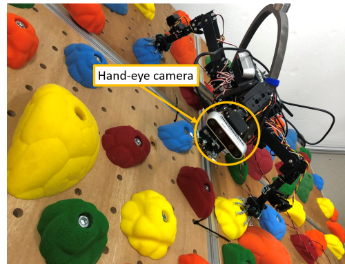
Fig. 1: Legged climbing robot platform: HubRobo equipped with a hand-eye camera.
