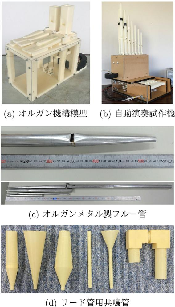
Fig. 2 これまでの試作事例. Examples of developed organ elements/models.
