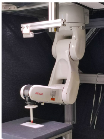
Fig. 8 紙に線を描く実験. Experiment that machine write a line on paper
