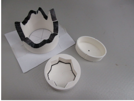
Fig. 9: 複雑な形状のファントム（トゲトゲ，楕円，多角形）. Complex-shaped phantom(spiny, ellipse, and polygon).
