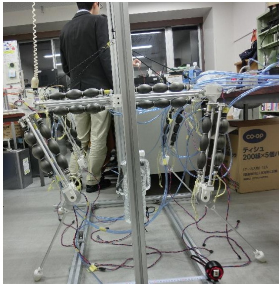
Fig.1 Hiyoshi's Four-Legged Walking Robot
