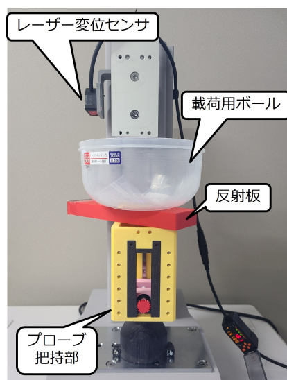
Fig. 9 機構作動検証 Verification of mechanism operation
