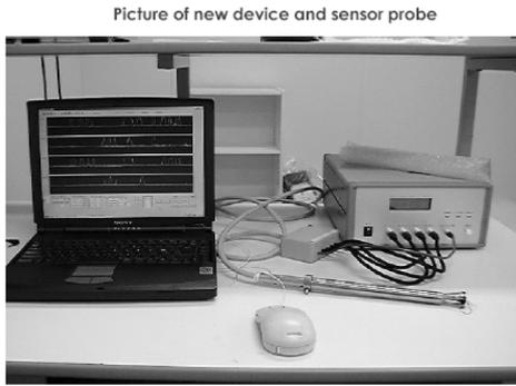
Fig.3 Picture of sensor probe and measuring system for the clinical evaluation of pelvic floor biomechanics.
