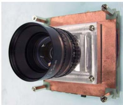
Fig. 1: An overview of the prototype camera.
