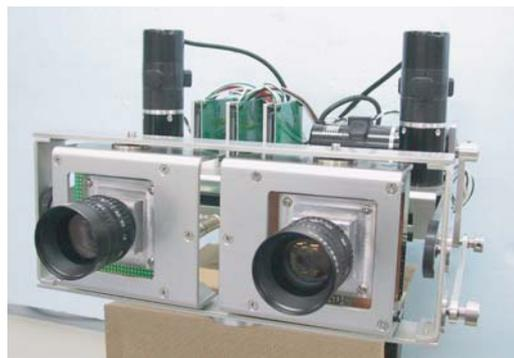
Fig. 4: An overview of the binocular camera head.
