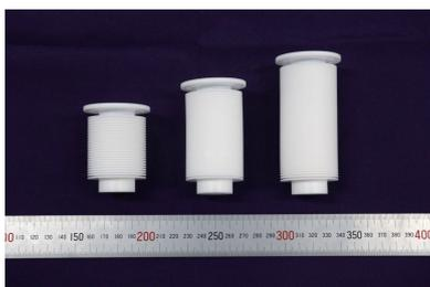
Fig. 3: Prototyped bellows with different number of pleats
