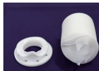
Fig. 7: Destroyed bellows after pressure resistance performance test
