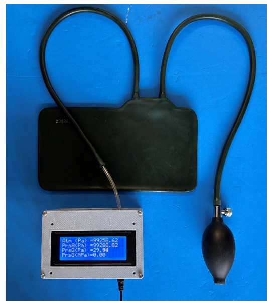
Fig. 7 腹腔内圧測定装置. Intra-abdominal pressure measuring device.
